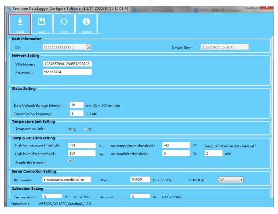
**3.** After modifying the parameters, for example, setting the WiFi account and password, click "Save" to save the interface parameter settings
