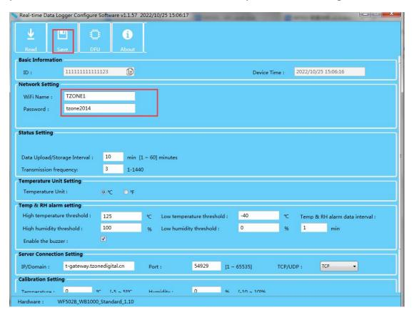
4. If you need to upgrade the firmware of the device, please click "DFU", and then upgrade according to our "Configuration Software Upgrade Step Manual"
