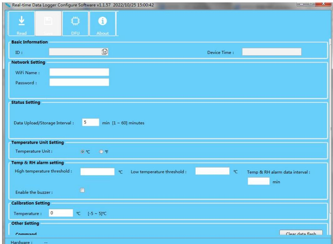
2. 点击“读取”可读取机器界面参数配置:
