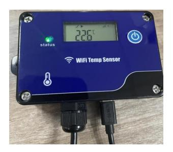
**Step3:** Connect the device to the computer by USB cable and click "Read" to read the device information (if the device cannot be read, please reconnect the USB cable.) Input the account and password of local WiFi in the "Network Setting" column -- click "Save" to save the configuration.
