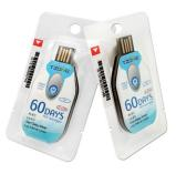
After getting the device, please don't tear the plastic bag but to quick press the button. If "ALARM" led and "OK" led flash at the same time, it indicates workable device. Otherwise, it's failure one and won't operate any more.
