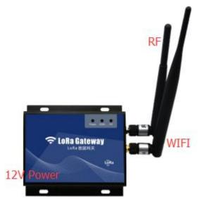
2.2 Turn on the device. (Left-on, right-off), The machine starts working when three LED lights flash at the same time.
