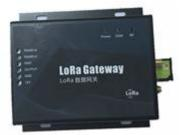
1.2 Install the RF and GSM antenna. Connect the device with the power supply.
