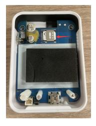
**Step2:** Install the 4G(LTE)/2G SIM card
