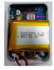
Step2: Install the 4G(NB/CAT-M1)/2G SIM card
