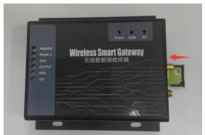
2.2 Install the RF and 4G antenna. Connect the device with the power supply.
