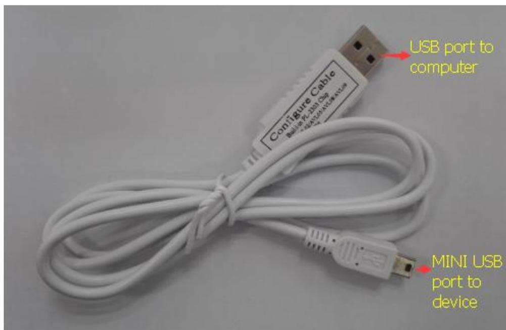
The RS232 cable is modified based on the normal RS232 Cable. It can be used to configure RD06 on personal computer.
