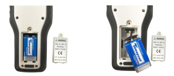
Step 1: Unscrew the screw and open the lid Step 2: Remove the battery
